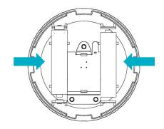
Install the two AAA batteries in the Sensor Housing with polarity as shown.
