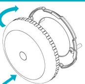
Install the Mounting Plate on an overhead surface using the two #6 screws provided. Place the Sensor Housing over the Mounting Plate, there is no "keyed" location. Rotate the Housing clockwise to lock it into place.
