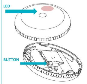
Test the Ceiling Motion Sensor from the desired location before permanently installing it by pressing the button twice to check network status.
