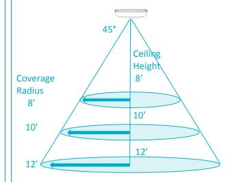
Position the Ceiling Motion Sensor for best use of its detection zones.
