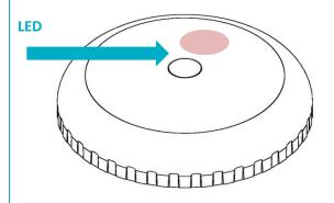
Verify that the device is sensing motion. The sensor requires a 3 minute "warm-up" time before it will report motion.
